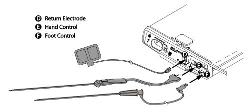
9. Connect the return electrode to the receptacle on the AEM Monitor.
