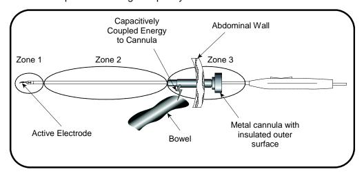
AEM instruments, in conjunction with an AEM Monitor properly connected to the electrosurgical generator (ESU), continuously monitor and dynamically manage "stray energy" (insulation failure and capacitive coupling) in zones 2 & 3.
