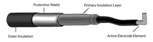
The AEM instruments incorporate a layered design. AEM instruments are shielded and monitored to prevent stray electrosurgical burns along the shaft of the instrument caused by insulation failure or capacitive coupling. The protective shield built into all AEM instruments provides a neutral return path for capacitively coupled energy and protection from insulation failure. The shield is continuously monitored during surgery which provides continuous assurance of the integrity of the instrument.
